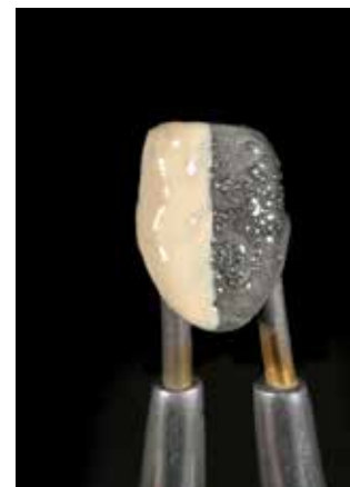
Easy mixing of O-base (1) and OA (2) to create A3 opaque color. Perfect masking properties of the framework.
