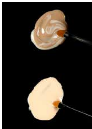
Easy mixing of O-base (1) and OA (2) to create A3 opaque color. Perfect masking properties of the framework.
