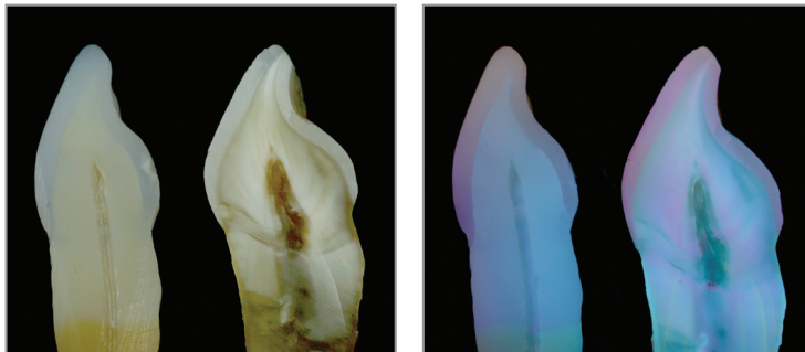
Mosaic composite specimen (A2 and EN) next to a natural human tooth under photographic light (left) and black light (right).
